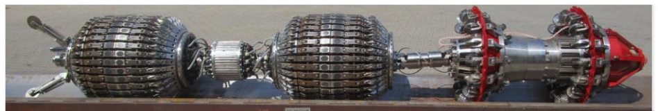
30" EMAT Ultra before the inspection
